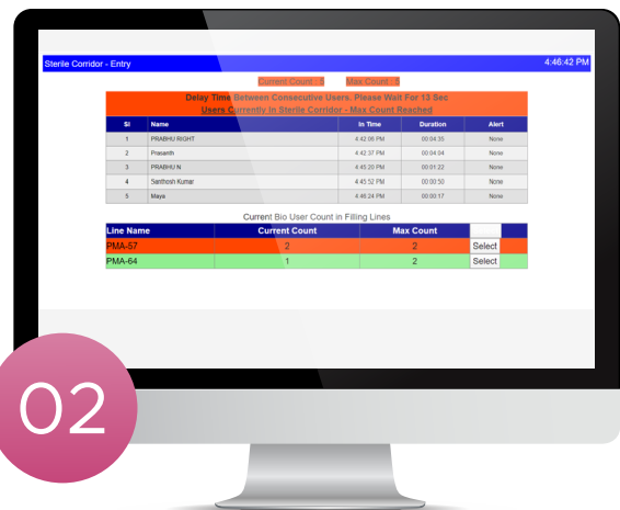
Entry HMI of Sterile Area Entry Door with multiple filling lines
